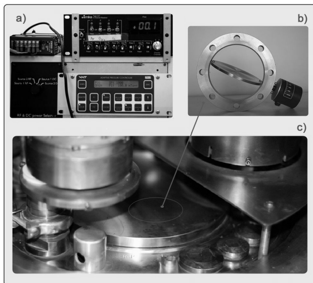
Fig. 1. Added instruments: MKS type 247D four channel readout and VAT PM3 pressure controller (a), butterfly VAT series 61 throttle valve (b), inside view of the sputtering system, new throttle valve is beneath a “Poppet” valve (in the ring) (c)
