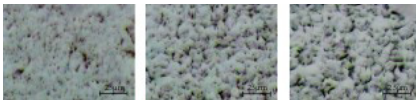
Fig. 3. Microstructure of undoped \text{Bi}_4\text{V}_2\text{O}_{11} sample (sintering time – from left to right 1 h, 5 h, 10 h)
