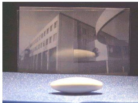
Fig. 7. Glare of a white object placed in front of aAS-AG coated plastic (left) and an uncoated one (right). The picture of the building placed 2 cm behind the substrates is clearly visible in both configurations
