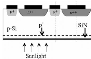
Fig. 2. Structure of an interdigitated back-contact solar cell
