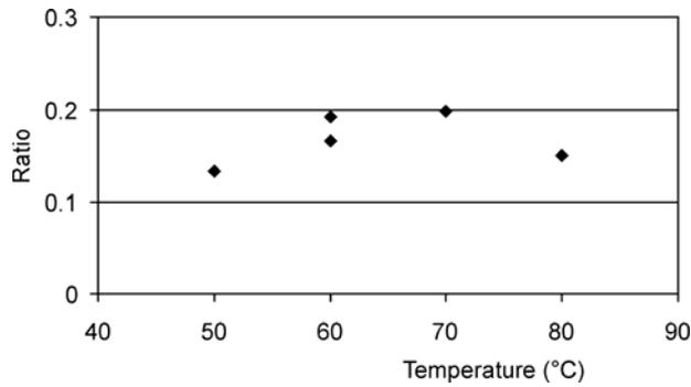
Fig. 4. The ratio of etching rates of (111) and (100) planes vs. temperature of solution: [TMAH] – 0.83%, [IPA] – 83%, duration – 3h
