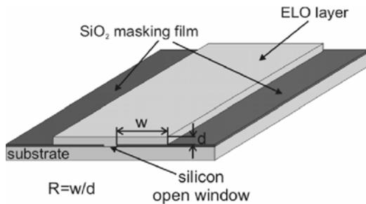
Fig 1. Schematic cross section of the ELO layer: the width  $w$  and thickness  $d$ , as well as the aspect ratio  $R$  of the ELO layer are defined herein
