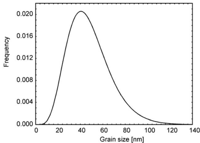
Fig. 1. Grain size distribution of Co<sub>3</sub>O<sub>4</sub> (sample P1)
