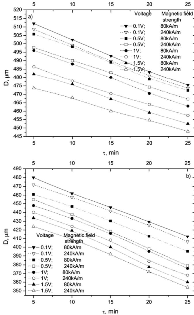
Fig. 7. Time dependences of the cylinder diameter  $D$  at the elevation of the quasi-periodic surface structure of the cylinder: a) under its cathode corrosion b) under its anode corrosion in the 7% solution of nitric acid. Mean error  $\sim 25\%$
