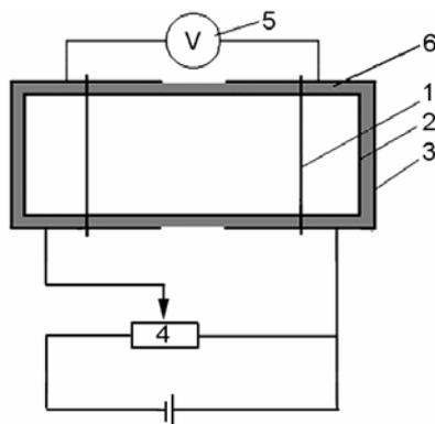
Fig. 1. The functional scheme of the electric circuit connected to the container with iron cylinders.
