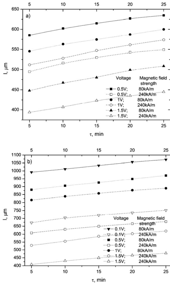
Fig. 5. Time dependences of the cavity length  $l$  of the quasi-periodic surface structure of the cylinder: a) under its cathode corrosion in 7% solution of nitric acid, b) under its anode corrosion. Mean error  $\sim 25\%$
