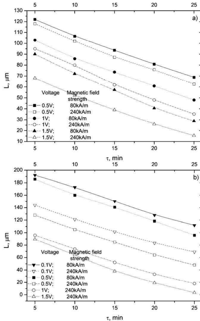
Fig. 4. Time dependences of the elevation length  $L$  of the quasi-periodic surface structure of the cylinder: a) under its cathode corrosion in the 7% solution of nitric acid, b) under its anode corrosion. Mean error  $\sim 25\%$
