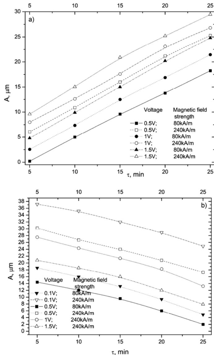
Fig. 6. Time dependences of the amplitude  $A$  of the quasi-periodic surface structure of the cylinder: a) under its cathode corrosion in the 7% solution of nitric acid, b) under its anode corrosion. Mean error  $\sim 25\%$
