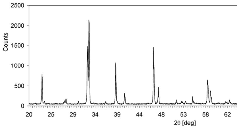
Fig. 6. XRD pattern for the  $YBa_2Cu_3O_{7-\delta}$  after sintering with sugar
