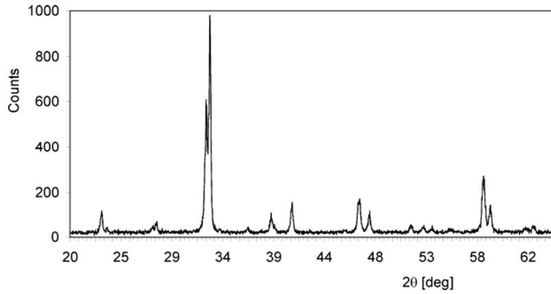
Fig. 5. XRD pattern for standard  $YBa_2Cu_3O_{7-\delta}$
