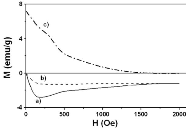
Fig. 4. Simultaneous measurement of two components ( $M_x$  and  $M_y$ ) vs. applied field: a)  $M_x$  (single flux state) along the  $x$ -direction ( $ab$ -plane), b)  $M_x$  (two flux condition) along the  $x$ -direction ( $ab$ -plane), c)  $M_y$  (two flux condition) along the  $y$ -direction ( $c$ -axis),  $H_{FC} = 1$  kOe and  $T = 77$  K
